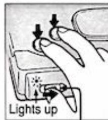
Slide the power switch (with the green button pressed) to the right, then release it.
