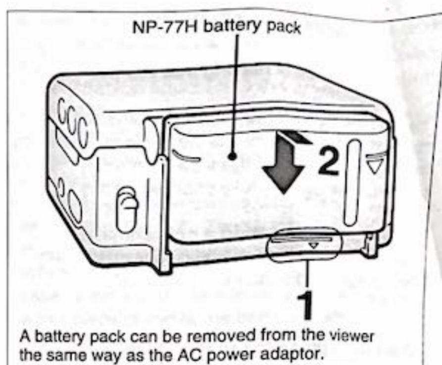
**1** Align the bottom of the battery pack with the line on the viewer.
